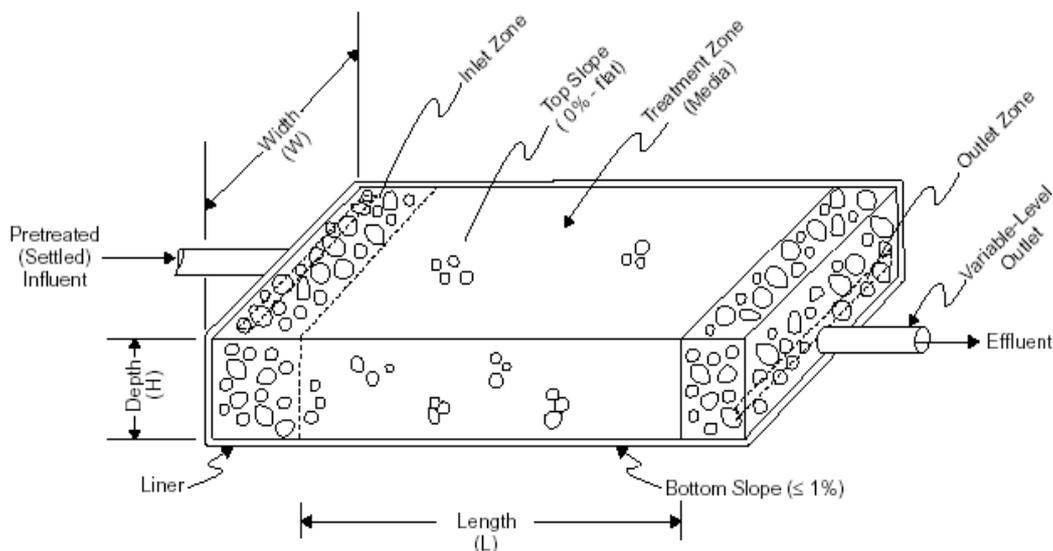
Fig. 4.2 Cross-section design of Constructed Wetland compartment
