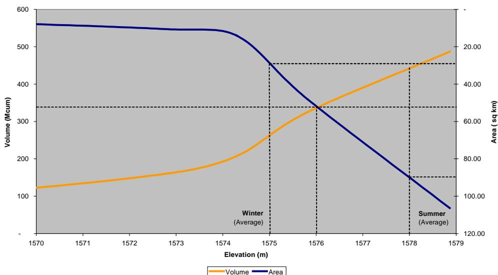
Fig 8 : Area Capacity curve for Wular Lake
